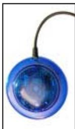
Classroom receivers capture the signals sent by the student transmitters. In a large classroom, utilizing multiple receivers to ensure that all student input is captured correctly is not uncommon. These receivers, usually mounted to a wall or ceiling, are connected by standard network cabling and terminate into a specialized hub that typically plugs into the USB or serial port on a personal computer or laptop. Software on the computer drives the
